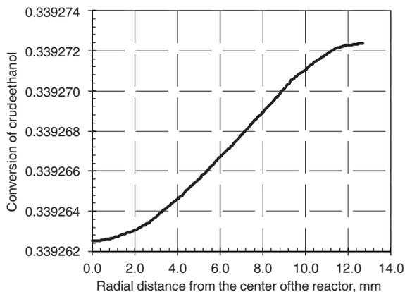
Fig. 8. Radial concentration profile of crude ethanol at a depth of 1.8 m from the top of the catalyst bed. The operating conditions and parameters used are presented in Table 1, column 4, for the hypothetical industrial crude ethanol reformer.
