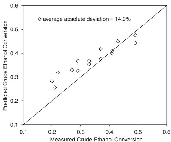
Fig. 4. Comparison of measured and predicted crude ethanol conversion within the temperature range from 593 to 793 K and WHSV range from  $4.67 \times 10^{-4}$  to  $1.28 \times 10^{-3} \text{ s}^{-1}$ .
