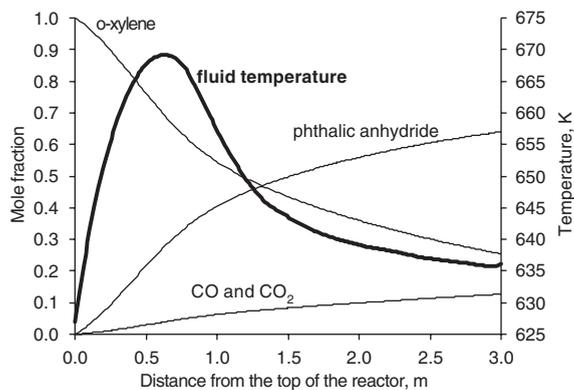
Fig. 2. Center line axial concentration and temperature profiles in multi-tubular *o*-xylene oxidation reactor (operating conditions and parameters are as presented in Table 3, column 5).
