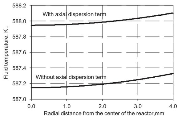
Fig. 7. Effect of axial dispersion term on the temperature profile at a depth of 30 mm from the top of the catalyst bed at a feed temperature of 593 K and  $W/F_{A0}$  of 2016 kg-cat s/kg-crude.
