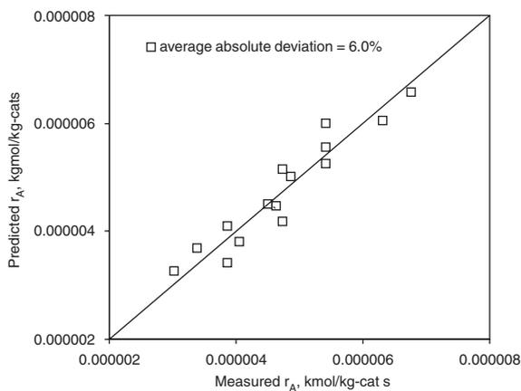
Fig. 3. Comparison of measured and predicted rates of reaction (mechanism based model of Eq. (9)) within the temperature range from 593 to 793 K and WHSV range from  $4.67 \times 10^{-4}$  to  $1.28 \times 10^{-3} \text{ s}^{-1}$ .
