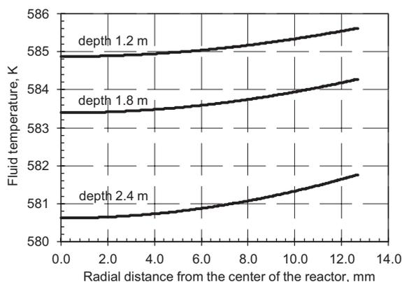
Fig. 9. Radial temperature profiles at various catalyst bed depths in the tubular reactor of the industrial crude ethanol reforming. The operating conditions and parameters used are presented in Table 3, column 4, for the hypothetical industrial crude ethanol reformer.
