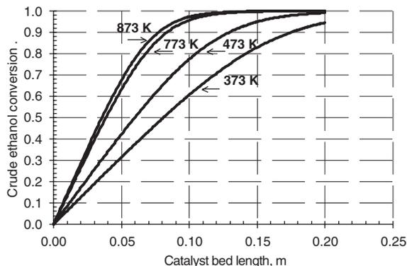
Fig. 10. Effect of catalyst bed length on crude ethanol conversion at various feed temperatures, catalyst bulk density of  $1126 \text{ kg/m}^3$  and  $W/F_{A0}$  of 2000 s.
