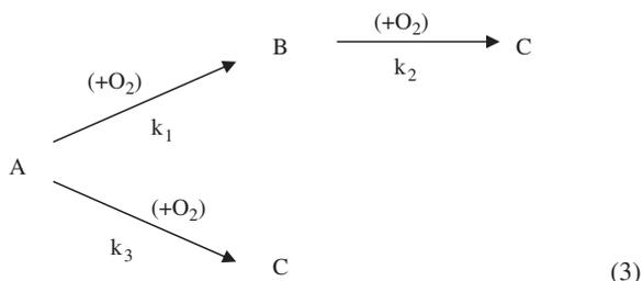
where A represents *o*-xylene, B represents phthalic anhydride, and C represents the total amount of carbon monoxide and carbon dioxide. Due to a very high excess of oxygen, the reactions can be considered to be pseudo-first-order, and the reactions kinetics can be described as in Eqs. (4)–(6) in terms of mole fraction:
