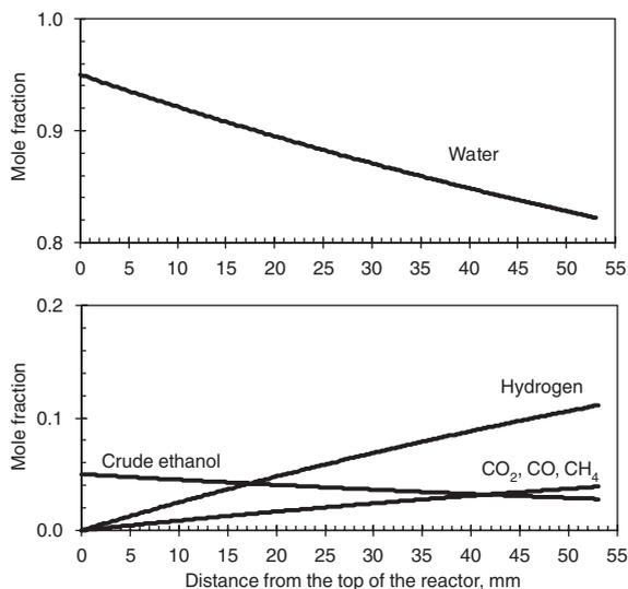
Fig. 5. Concentration profiles along the reactor at a feed temperature of 593 K and  $W/F_{A0}$  of 2016 kg-cat s/kg-crude.
