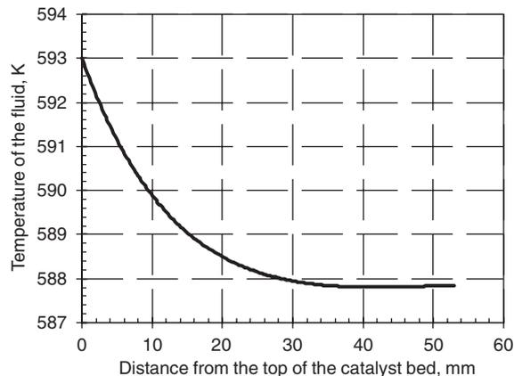
Fig. 11. Axial temperature profile of the fluid along the center of the tubular reactor at  $W/F_{A0}$  of 2016 kg-cat s/kg-crude and inlet feed temperature of 593 K. The parameters used are presented in Table 1, column 3.
