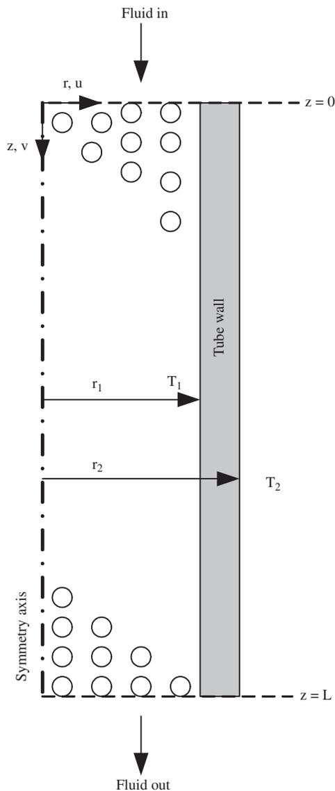
Fig. 1. A schematic diagram of the packed bed tubular reactor (PBTR).
