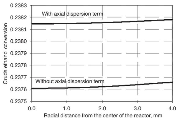
Fig. 6. Effect of axial dispersion term on the crude ethanol conversion profile at a depth of 30 mm from the top of the catalyst bed at a feed temperature of 593 K and  $W/F_{A0}$  of 2016 kg-cat s/kg-crude.
