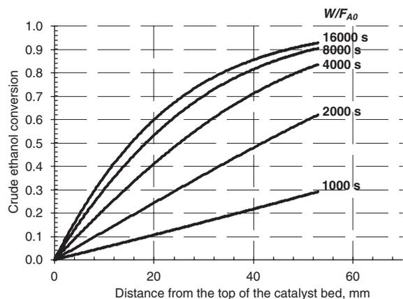
Fig. 12. Effect of  $W/F_{A0}$  on crude ethanol conversion in the axial direction at 693 K and bulk density of  $1126 \text{ kg/m}^3$ .
